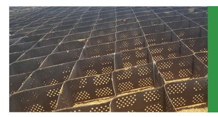
ForCell is a 3D geosynthetic material in honeycomb shape which is manufactured by ultrasonic welding of adjacent PE perforated strips allows drainage between neigbour cells.
