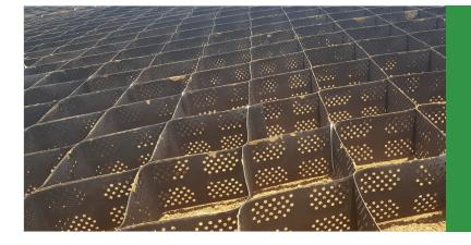
ForCell is a 3D geosynthetic material in honeycomb shape which is manufactured by ultrasonic welding of adjacent PE perforated strips allows drainage between neigbour cells.
