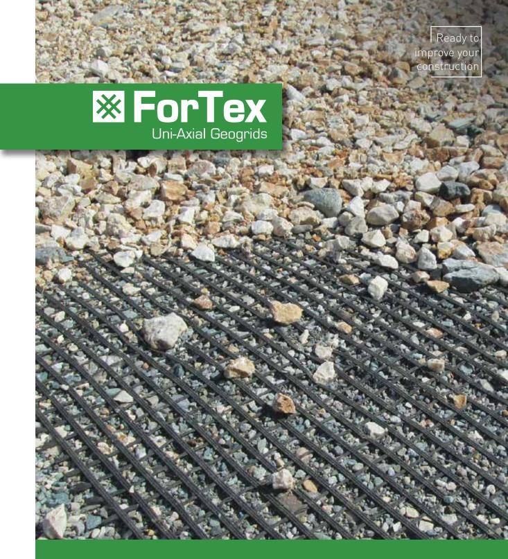
ForTex Uni-Axial Geogrids are high-strength materials which are manufactured by knitted polyester yarns in rectangular form and covered with polymeric coating, developed for uni-direction geogrids requirements for various applications of civil engineering.
