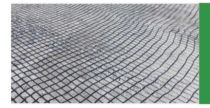
ForTex GG products are geogrids which are composed of knitted and woven polyester yarns in rectangular shape and covered by polymeric base coating.
