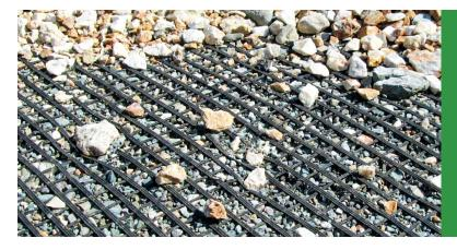
ForTex GG products are geogrids which are composed of knitted and woven polyester yarns in rectangular shape and covered by polymeric based coating.
