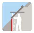
Bottom-operated centre-pivot roof windows are recommended when high installation is required, for instance in connection with a high knee wall.
