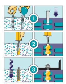
Two-components polyester adhesive used for anchoring under predominantly static loads
