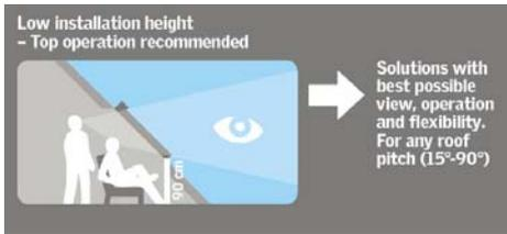
Top-operated centre-pivot roof windows make it possible to place furniture directly below the window without obstructing operation of the window.
