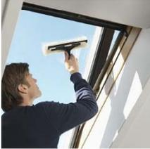
To clean the outer pane from the inside, rotate sash and secure in cleaning position with barrel bolt.
