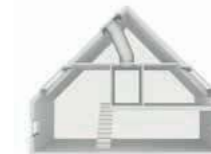
A tunnel of highly reflective coating inside carries daylight and moonlight up to 6 meters from a discrete roof window - into the room beneath. Ideal for small rooms and tight spaces.
